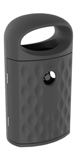
Litter bin made of 4mm thickness high density polyethylene. Rough and forge black finish. Resistant to UV rays, chemical agents and impacts. Stainless steel cigarette stubber. AISI 304 stainless steel screws.
