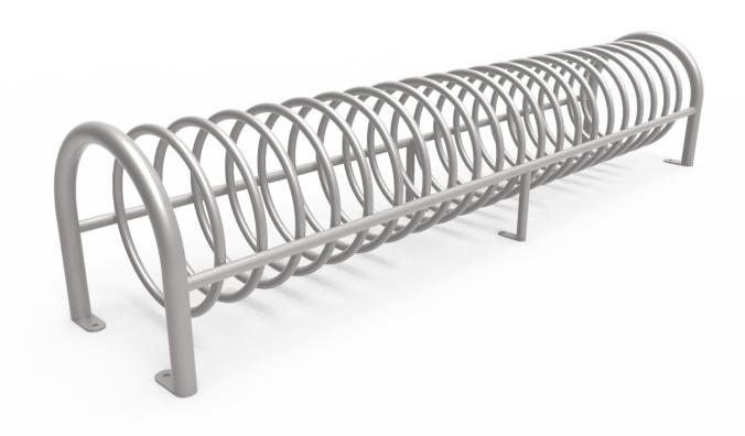
Bike rack made of electro-galvanised steel with epoxy primer coating and grey RAL 9006 polyester paint coating. Recommended anchoring: four M8 expansion bolts depending on the surface and project.
