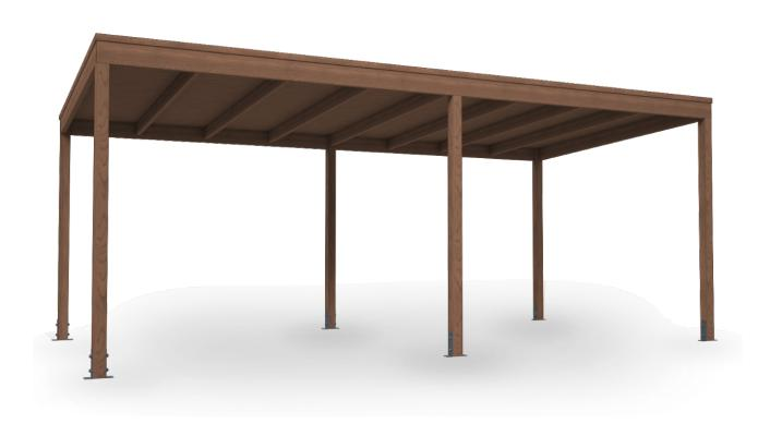
$6000 \times 3000 \text{ mm}$  self-supporting gable roof pergola made from European Oregon (Douglas) pine.  $90 \times 90 \text{ pillars}$ ,  $170 \times 45 \text{ beams}$ ,  $140 \times 45 \text{ joists}$  and  $115 \times 21 \text{ tongue-and-groove boards}$ . Lasur coating, 100% natural vegetal oil- and resin-based varnish finish with a protective UV overcoat in golden oak colour.
