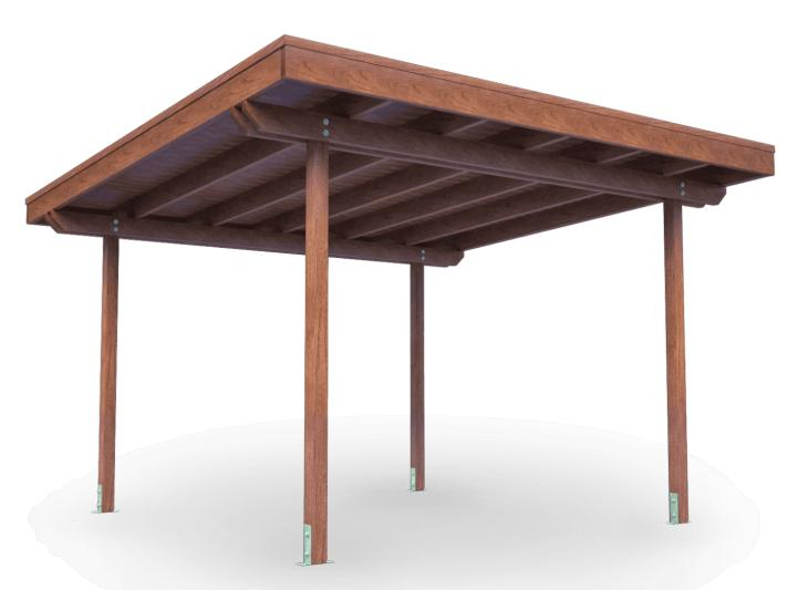
4000 x 4000 mm gable roof pergola made from European Oregon (Douglas) pine. 90 x 90 pillars, 140 x 45 beams, 100 x 45 joists and 115 x 21 tongue-and-groove boards. Lasur coating, 100% natural vegetal oil- and resin-based varnish finish with a protective UV overcoat in golden oak colour.
